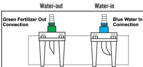
No pipe cutting required with saddle connection
